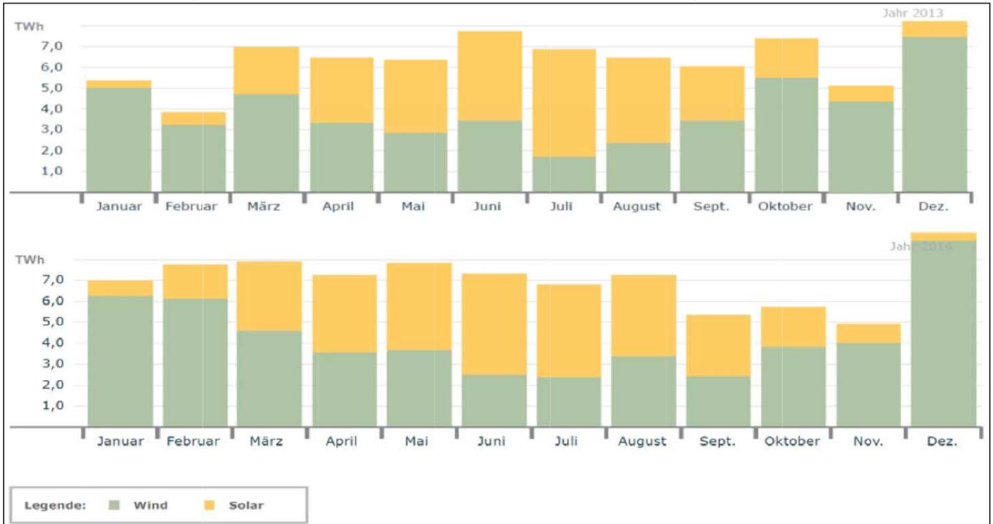
Monthly power production from PV and Wind in Germany (2012 and 2013)
